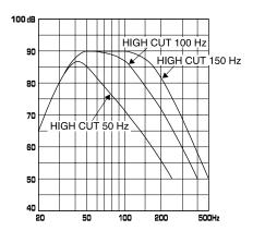
The figures below show the optimum adjustment of each control and the frequency characteristics when this subwoofer is combined with a typical main speaker system.
