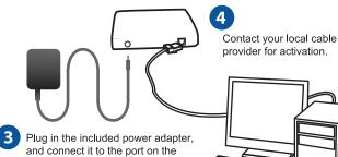
rear of the CDA-30360, and connect an Ethernet cable from the RJ-45 port on the CDA-30360 to your computer or router.
